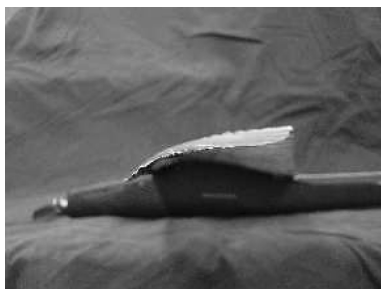
Fig. 4 Side view of the MAV with a) negative, b) neutral, and c) positive morphed wing.
