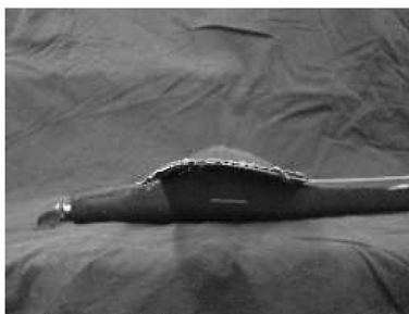
Fig. 4 Side view of the MAV with a) negative, b) neutral, and c) positive morphed wing.
